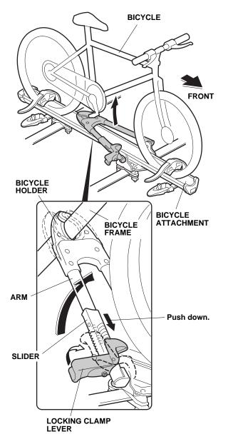
13. Push up the locking clamp lever to secure the bicycle frame.
